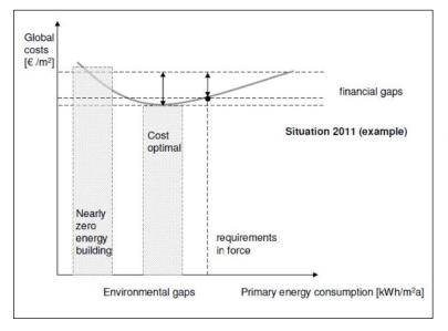
Figure 8: Example: Financial and environmental gaps between nearly zero-energy building, cost optimality and current requirements in 2011
