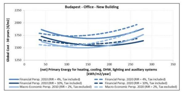
Figure 9: Impact of assumed changes between 2010 and 2020 on crucial input parameters – Budapest – Office - New building
